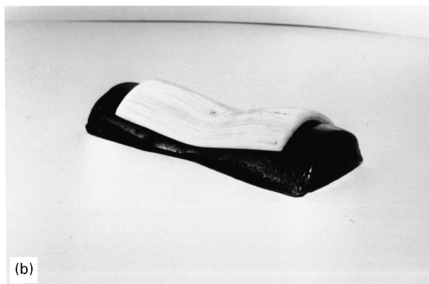
Figure 9 GF/EP [0]6 saddle samples and their corresponding models, (a) right model on Fig. 6; (b) left model on Fig. 6.
