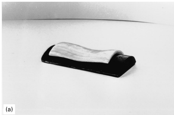
Figure 8 Effect of silicon rubber pad thickness on surface quality of saddle composite samples. Pad thickness: (a) 0; (b) 1 mm; and (c) 2.5 mm.
